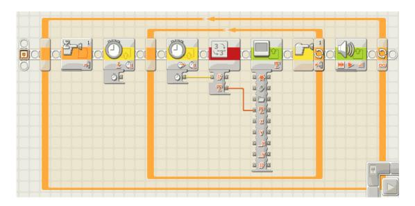
The program consists of two loops, an outer and an inner loop. The outer loop makes the program run forever. This way, the stopwatch can be used to measure several time intervals in a row without having to restart the program.
