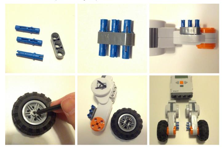
Finally, connect the wheels to the NXT. Make sure the cables are plugged in port B and port C of the NXT.
