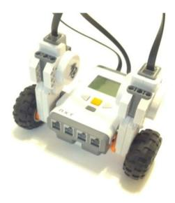
First, assemble a pole that acts as a "3rd wheel" to balance the robot.
